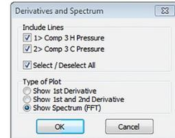
Above the pressure data, a frequency analysis of the pressure signal is provided to the user. By implementing smoothing factors one step at a time, the effect on the pressure FFT is shown. The goal is to reduce the high frequency peaks that are caused by indicator resonance, but to not affect the lower frequency pressure. As the smoothing factors are increased, the high frequency peaks will drop, as shown below.
