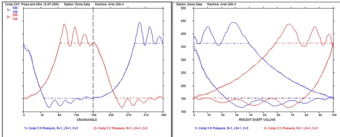
The above pressure-time and pressure-volume traces show high indicator channel resonance which is typical for high-speed compressors. Windrock MD software provides two methods to determine the amount of smoothing required to eliminate this problem.
