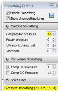
If too much smoothing is implemented by the user, the low frequency pressure curves may be affected or new high frequency peaks may appear. Fortunately, Windrock MD provides a warning to the user if excessive smoothing is added.
