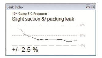
In this example of a slight suction and/or packing leak, notice the slope of this line is going down, indicating the mass quantity of gas is decreasing during compression. Since there is only a  $\pm 2.5\%$  change, this is not as critical as if it were a higher percentage leak.
