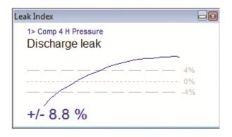
In this discharge leak, notice the line is sloping upward, indicating the mass quantity of gas increasing during compression. In an ideal cylinder with no leaks, the mass would be constant throughout the cycle. But here, the mass quantity changes by 8.8% in each direction (17.6% total).
