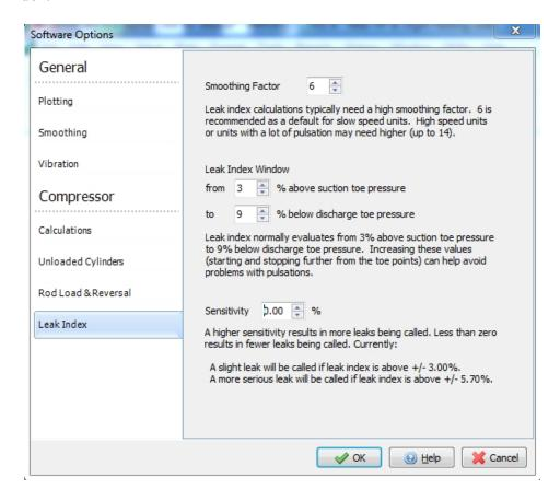
The Leak Index is a proven feature that helps make Windrock MD software the most advanced reciprocating analysis software available. It is available for our portable analyzers, as well as our online systems. Our Technical Services Team always utilizes Leak Index when analyzing equipment.
